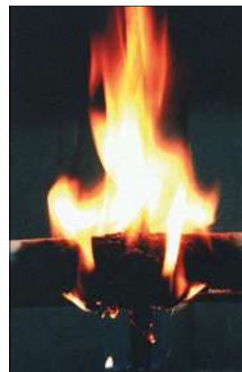
Mancata espansione del prodotto installato in ambiente umido Failure to expand the product installed in a humid environment
