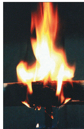
Mancata espansione del prodotto installato in ambiente umido Failure to expand the product installed in a humid environment
